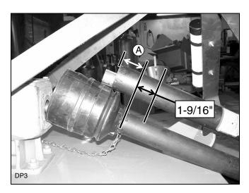
Figure 6. Determine Shield Length
